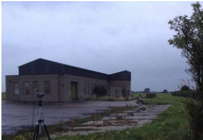
Viewing a scene using a camera observing a Rotakin Test Target
