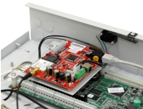
Figure 8: a dual transmission path (Ethernet/GSM) supervised premises transceiver (in red) mounted inside a control panel.
