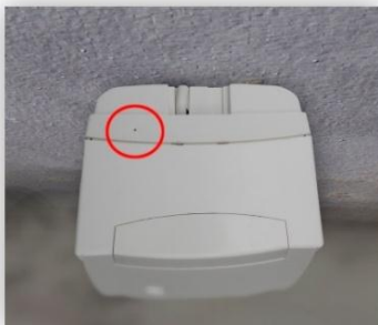
Figure 11: Check for small holes
