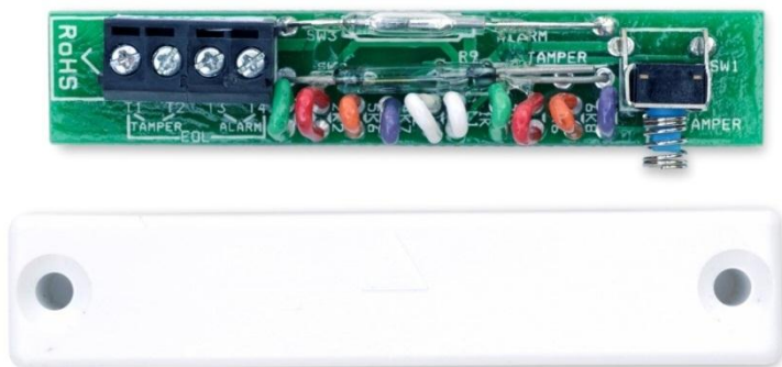
Figure 48: Selectable end-of-line resistor combinations. The coloured wire links inside the protective switch allow for the selection of end-of-line resistors matching the CIE configuration to provide a supervised interconnection.
