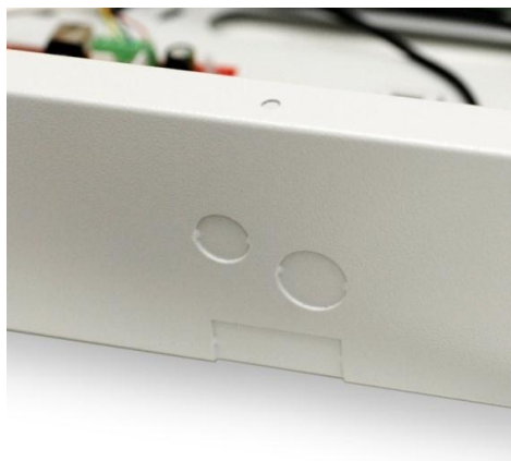
Figure 9: Unused cable entry/conduit knock-out points with blanking plates intact
