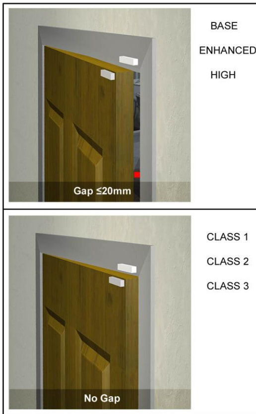
Figure 47: Acceptable range of opening movement
