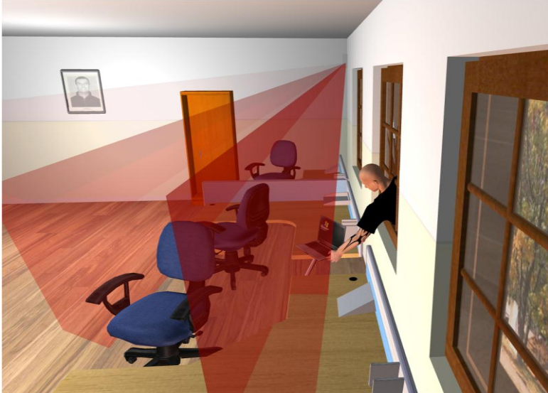
Figure 20: Assets placed close to a window may not be protected
