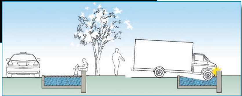
Figure 4-47: Planting cover layer creates a TigerTrap planting with a rear bench. SOURCE: ROCK 12 SECURITY ARCHITECTURE
